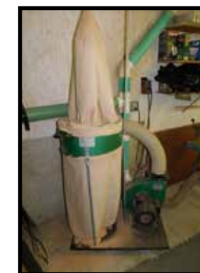
Dust collector, 70 gal. 2 hp
