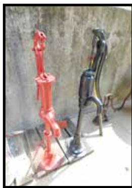
Cast iron yard water pumps
