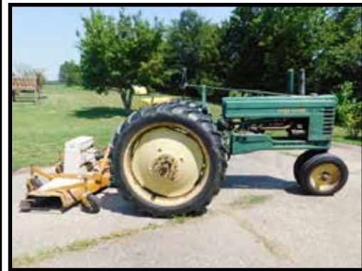
1945 John Deere B gas tractor w/add on 3 pt hitch & PTO, 11.2 -38 tires, extra clean, runs good
