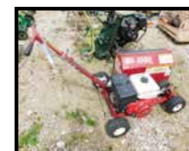
Brown bed edger, trencher, Model F990H, 9 hp, Honda
