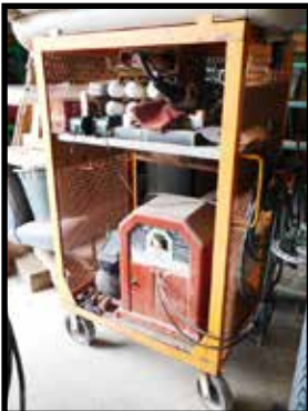
Lincoln AC 225 – S welder
