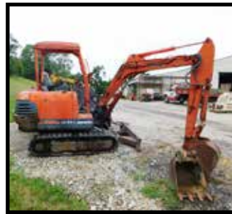
Kubota KX91-2 track hoe w/rubber tracks, diesel w/two pattern selection system
