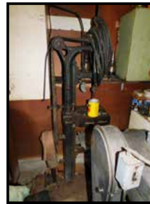
Belt driven, floor model drill press
