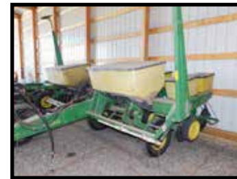
John Deere 7000 planter, 4 row w/fertilizer & insect boxes
