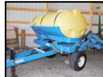
J&M Innovation, pull type, anhydrous applicator w/600 gal. tank
