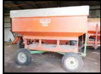
3 Flickin Model 231, gravity flow grain wagons on Lindsay running gears
