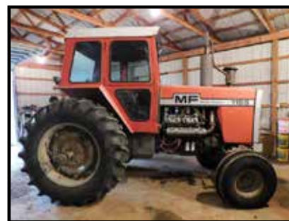
1978 Massey Ferguson 1155, diesel tractor w/cab & air, 20.8-38 tires & duals, dual hydraulics, 3452 hrs. extra clean
