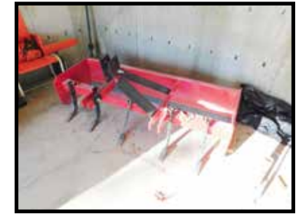
Mahindra HD-B-6, 6' box scraper set, new TB-70, 70 1/4" WR long bolt on tooth bar
