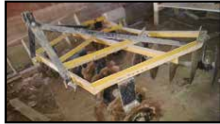
King Kutter 3pt., 6 ft. (notched front blade) disk
