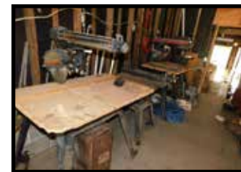
Craftsman 12" radial arm saw, floor model
