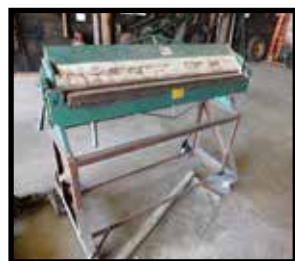
Tin Knocker Model 2248, 22ga, metal shear
