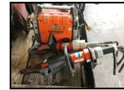
Holmatro w/Honda engine, 10,000 PSI pump
