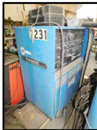
Miller Syncrowave 350 for Tig welding, CC-AC/DC welding power source
