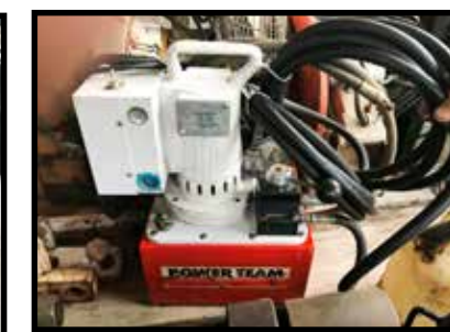
Power Team 1 1/8th hp, 12,000RPM, 115 volt, 20 amp cycles, 60/50 AC
