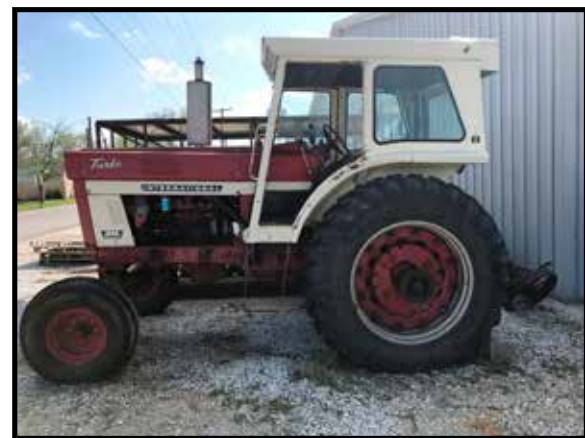
1975 IH 1066 diesel Turbo, wide front-end, 3-pt. hitch, dual hydraulics, 18.4-38 tires w/hubs, 540 & 1000 PTO, shows 8,382hrs.
