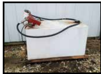
100-gal transfer tank w/12-volt pump
