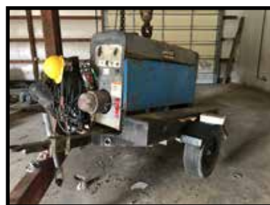
Lincoln arc welder power plant, SA 200 w/single axle trailer
