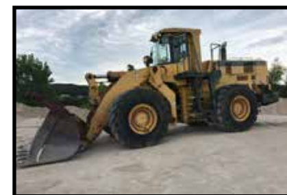
Komatsu Model WA 600-3L with 12' bucket, good unit, SN 52097
