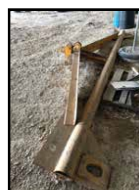
40-ton gin pole
