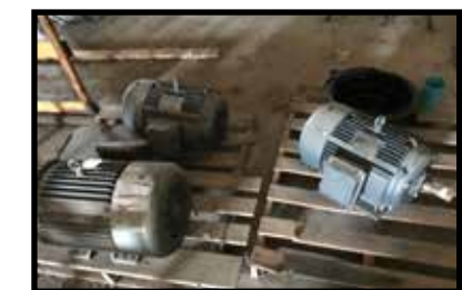
2 new 20hp, 3-phase motors
