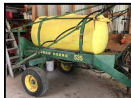
John Deere #535 boom sprayer, approx. 350gal, trailer-type, approx. 30' booms
