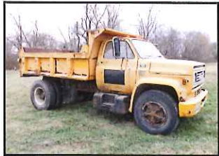
1977 Chevy C-65 dump truck, 4 speed w/2 speed axle, 366 gas engine
