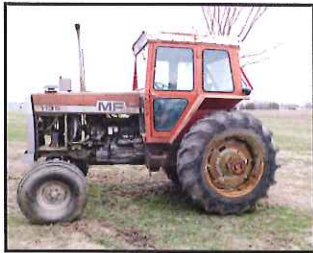
1135 Massey Ferguson, diesel tractor w/cab, 20.8-38 tires, shows 37xx hrs
