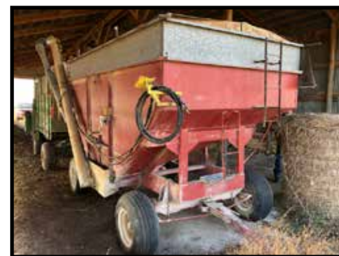
Seed tender, 275-300bu. electric running gear, hydra fold auger, homemade tarp
