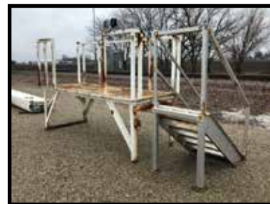
Metal barrel or fueling steps & platform
