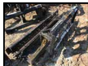
6' pulverizer for skid loader or 3pt
