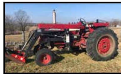
Farmall 826 diesel tractor, wide front-end, 3pt hitch, power steering, open station, 92hp, 540 & 1000 PTO, shows 5300hrs.
