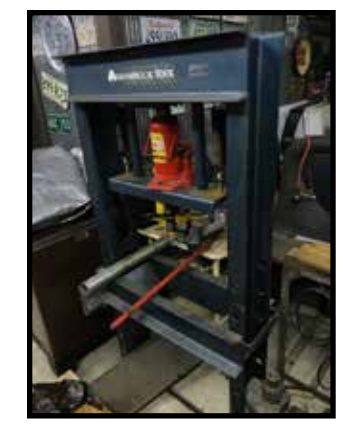
Floor-model 20-ton press
