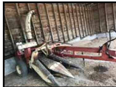
Hesston 7140, 2 row 30" direct cutter silage head with sharpener
