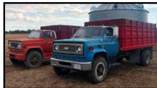
1979 Chevrolet C-70 grain truck, single axle, 5&2 transmission, 366 gas with 16' Knapheide grain bed & hoist (like new tires)
