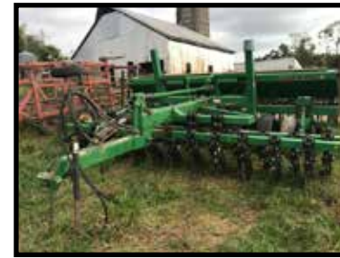
Great Plains solid stand grain drill with Great Plains 1500 center pivot no till caddy, 24 hold, 7 1/2" spacing
