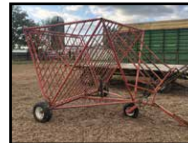
Square baler accumulator with hydraulic dump
