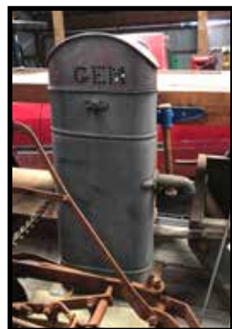
Gem cistern pump
