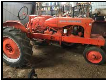
AC 1939 RC tractor, narrow front end, 12.4-26 tires, RC rear end, SN 1016
