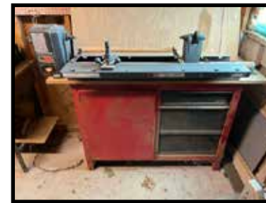
Craftsman 12" wood lathe, spindle feed with base cabinet
