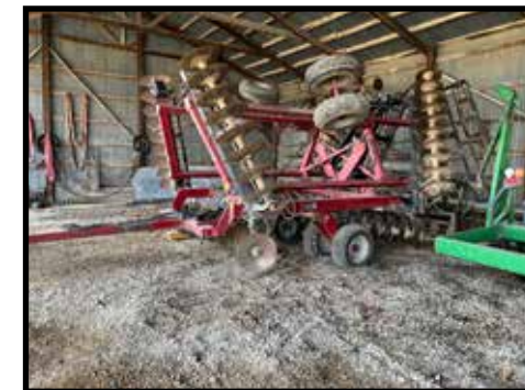
Case IH #496, 22'9" front cut w/Remlinger 25' roller basket, (9" spacings & 20" blades) kept shedded, good disk
