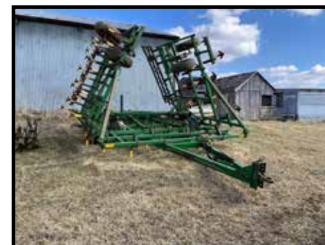
John Deere #960, 31' pull type field cultivator w/coil tine harrow, approx. 300 acres on new shovels
