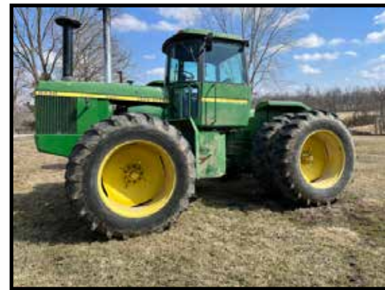
1977 John Deere 8430 articulating, 4 wheel drive, with cab, 3 pt. w/Quick Hitch, 3 hydraulics, big 1000 PTO, 18.4-38 duals, shows 4371 hrs.
