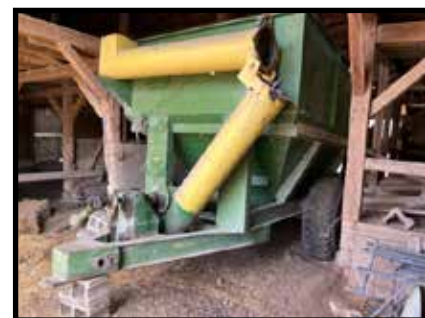
John Deere #1210 grain cart, 400 bu., w/manual fold auger & gate
