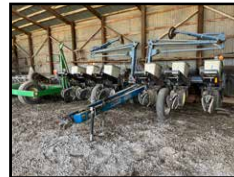
Kinze #2200, 12 row, 30" manual fold planter w/bean & corn meters & monitors
