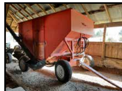
275 bu. Gravity Flow wagon w/Killbros 14' auger, used for seed wagon
