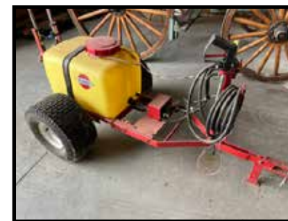
Hardi 30-gallon boom type, pull type sprayer
