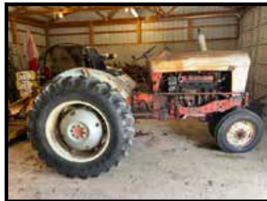
Ford 900 gas tractor w/tricycle front end, 3 pt. w/PTO, like new 13.6 - 28 tires, shows 1910 hrs.
