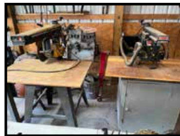
7730 DeWalt power shop radial arm saw, 2 hp., 250mm w/ 10" blade
