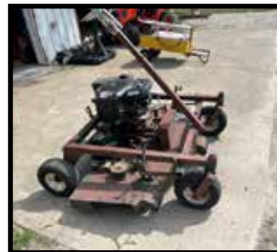
Swiss pull type 5 ft. finish mower with twin 18 engine
