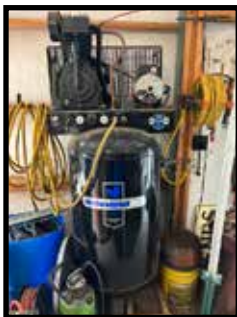
80 gallon 2 stage 5 hp industrial, 175 max PSI air compressor
