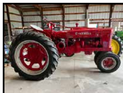
Farmall H with PTO, hydraulics & draw bar hitch, SN FBH359320 X1, restored
