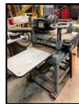
Delta DC 380 15" planer, floor model, with new set 15" blades
