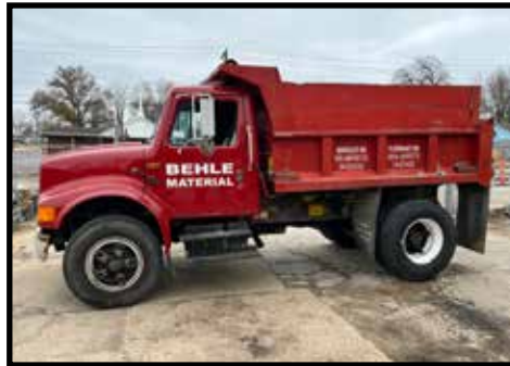
1991 International 4700 diesel dump truck, 5 speed w/2 speed axle, 10 ft. bed, 36,000 lb., with hydraulic bed, 11R22-5 tires, bought new, shows 81, xxx actual miles
