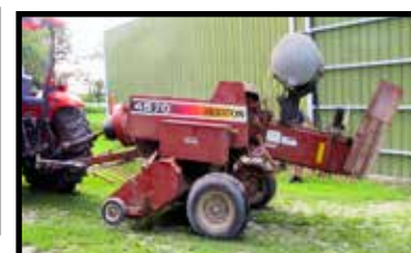
Hesston 4570 inline string tie hay baler w/acid attachment
