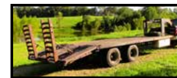
Homemade 20ft. gooseneck flatbed trailer 8' wide w/4ft. dove tail + ramps tandem axle (oil bath axles)
