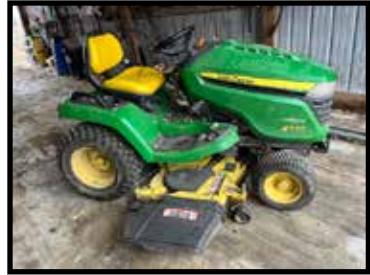
John Deere X530 multi terrain riding lawn tractor, 24 hp w/54 inch deck
