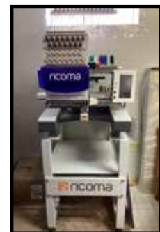
Ricoma embroidery machine, Model RCM-1501TC, 7S includes hoops, tools, 2 cap embroidery attachments, thread & hats
