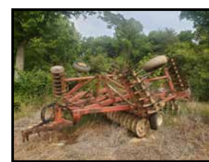
IH 22' hydraulic fold wheel disk, 21" blades & harrow attachment
