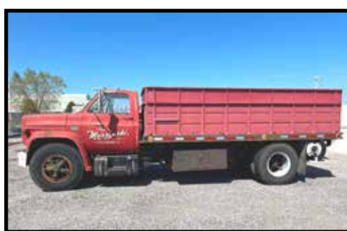
1975 Chevy C-60 grain truck w/Midwest 15'6" grain bed & hoist
