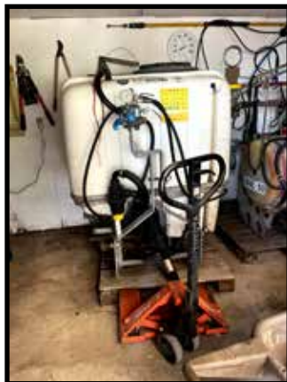
600 gallon PTO type orchard sprayer w/Durand Wayland Spraying System
