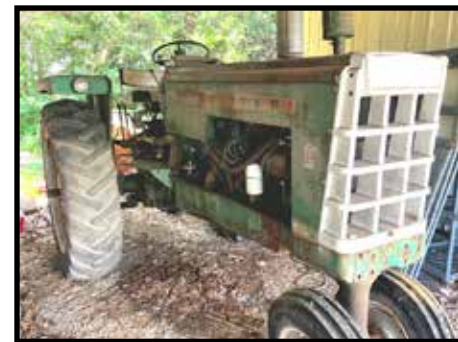
1963 Oliver 1600 gas open station, 6 cylinder, tri front end, 3 pt. w/PTO, power steering, 15.5-38 tires
