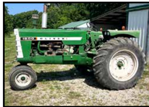
1960 Oliver 1800, 6 cylinder gas tri front open station, 3 pt. w/PTO, power steering, 18.4-34 tires
